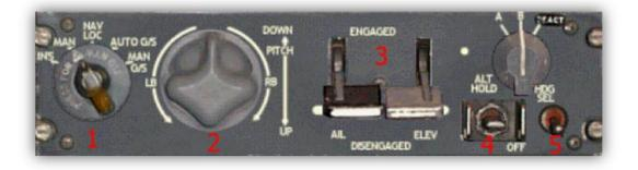
The Autopilot control unit is located in the radio stack, lower right side of the captain. There are 2 knobs, 2 levers and 2 switches that operate the SP-50.
