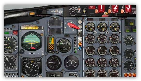
Start to advance the throttles to 60% and watch out for failures. After a few seconds, throttle up until EPR readings match the orange bugs you've already set. Build up some speed, and slowly rotate at 145 KIAS. Do not pull up very fast, the 727 is not a fast climber. You must build up speed first.
