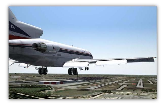
**IMPORTANT**: **DO NOT FLARE** the B727. This aircraft was not designed to flare upon touchdown. Instead, keep a steady approach speed; get the nose up 2 or 3 degrees, and the plane will land itself, nice and easy. If you flare, most likely you will float, lose airspeed and smash back on the ground; all that if you don't tail strike first.
