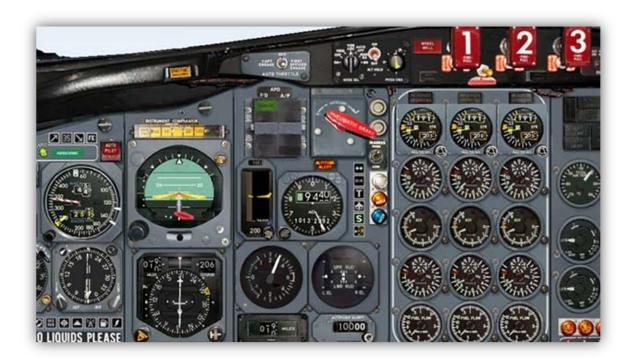
Before reaching the CHCLL intersection, you should be very close to 10,000 ft, our first level-off altitude, and aligned on the radial. Slowly decrease your vertical speed, and maintain 10,000 ft. Turn off the necessary lights, adjust your thrust and accelerate to 310 KIAS.
